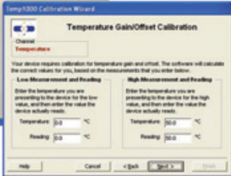
Figure 9: Software calibration adjustment to a logger
